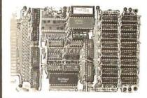
PET INTERFACE KIT—CONNECTS THE 32K RAM BOARD TO A 4K OR 8K PET. CONTAINS: INTERFACE CABLE: BOARD STANDOFFS. POWER SUPPLY MODIFICATION KIT AND COMPLETE INSTRUCTIONS. \$49.00
