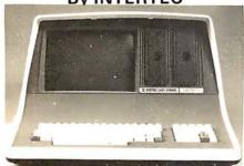
32K or 64K (Double or Quad Density units available). Uses two Z-80 CPU's. Commercial-type terminal with 12" monitor. Dual double density minifloppies. Over 350 kilobytes of storage (twice that with quad density drives). Two serial RS232 ports, I/O ports standard. Expandable with optional S-100 S-100 interface. Comes with CP/M<sup>TM</sup> 2.2 operating system. MiniMicroMart includes BASIC interpreter and can supply a wide range of CP/M Development and Application software.
