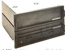
A 64K complete computer with dual density floppies (1 megabyte). Rack or vertical mounting. Systems with double-sided drives, hard disks, and multi-user (MP/M).
