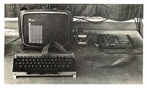
Photo 6: The complete terminal system with keyboard, monitor, power supply, and main circuitry.
